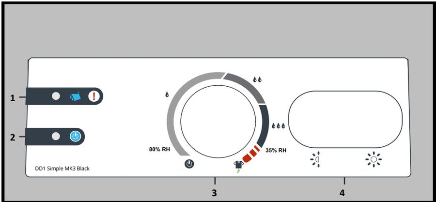
1. **Water Full/Check Indicator**
