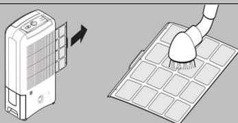
1. Turn off and leave for 5 minutes, then unplug the dehumidifier. Remove the filter.
