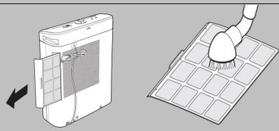
1. Turn off and leave for 5 minutes, then unplug the dehumidifier. Remove the filter.
