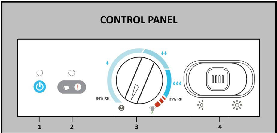
1. **Power ON Indicator**
